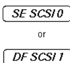
Figure D-28 SCSI Device Label for Devices with Restricted Space on the Front Bezel
