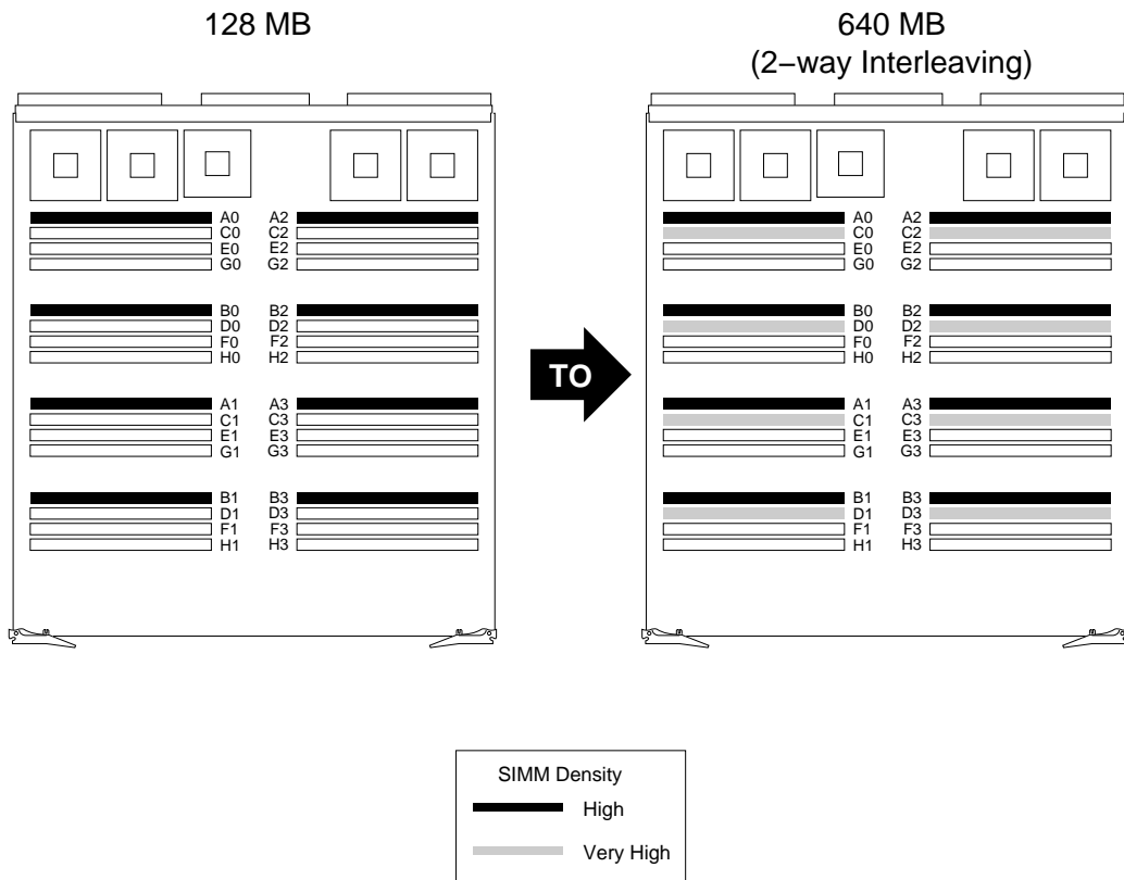
Figure C-14 128 MB to 640 MB (Two-way Interleaving)
