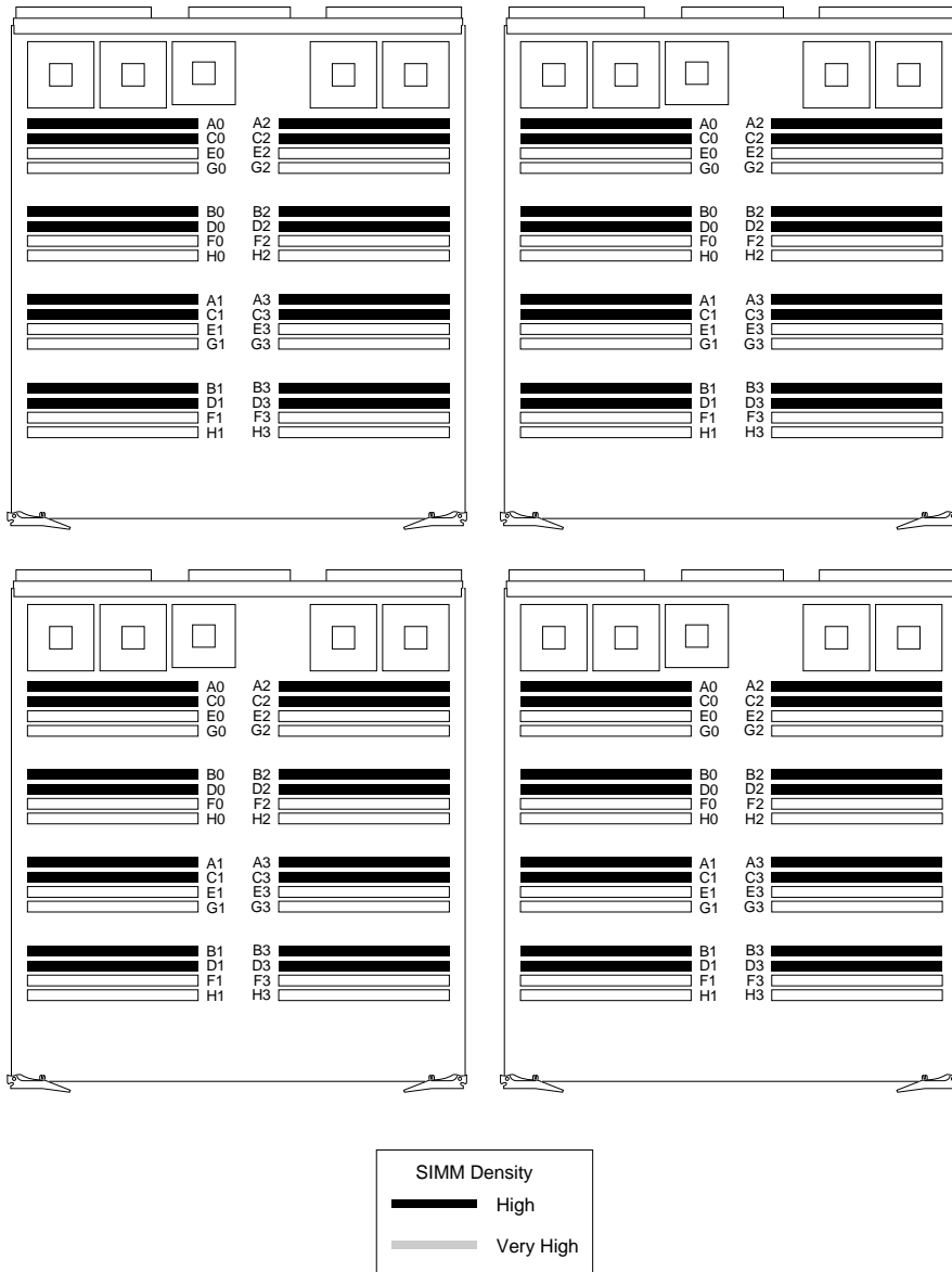
Figure 5-61 1024 MB Configuration (Eight-way Interleaving, Four MC3 Boards)
