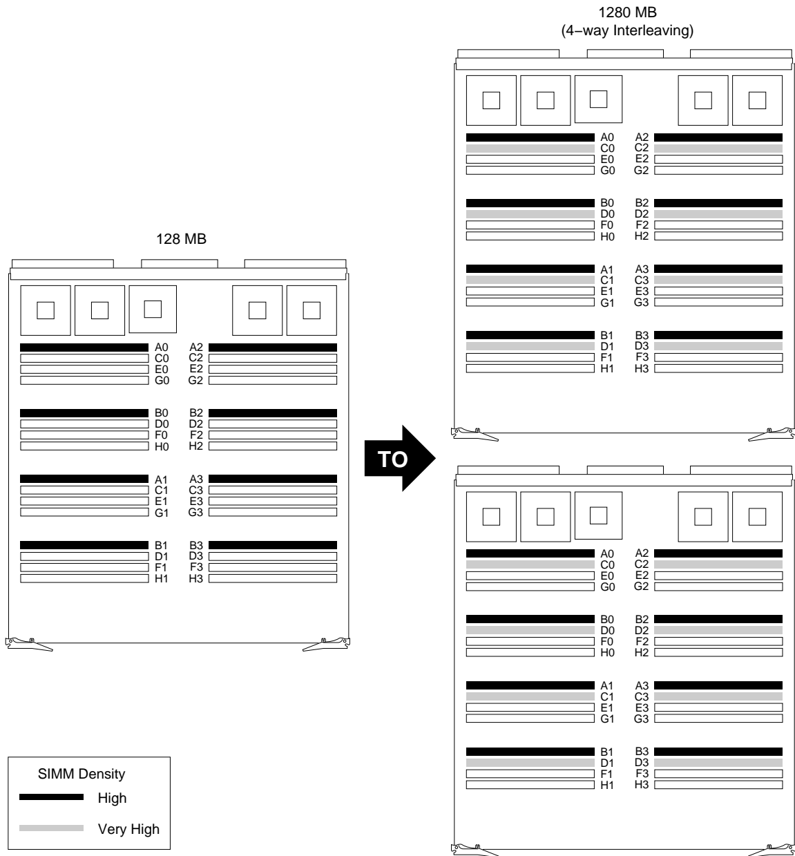
Figure C-16 128 MB to 1280 MB (Four-way Interleaving)
