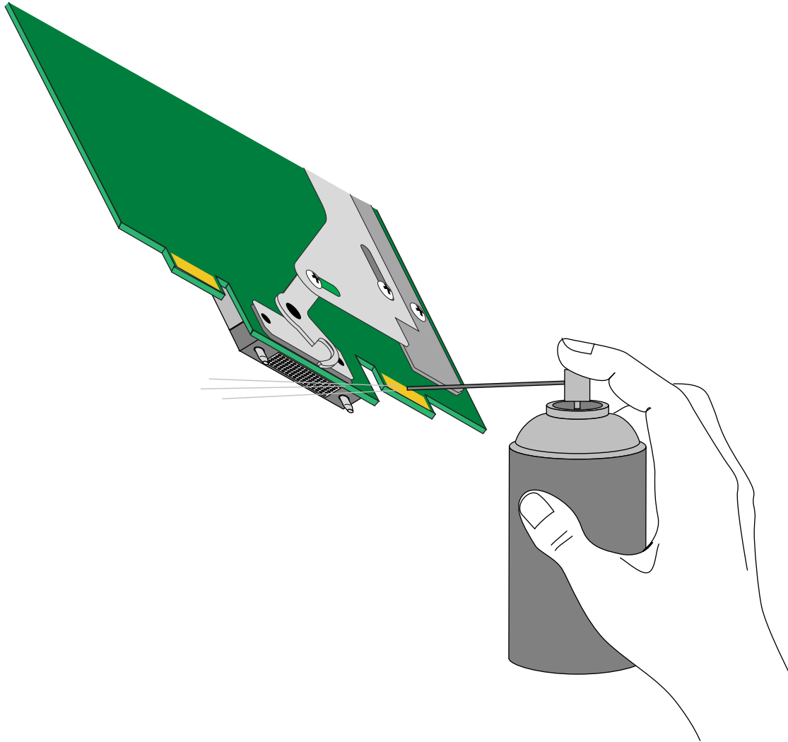
Figure 1-3 Position for Compressed Air Can When Cleaning Compression Connector
