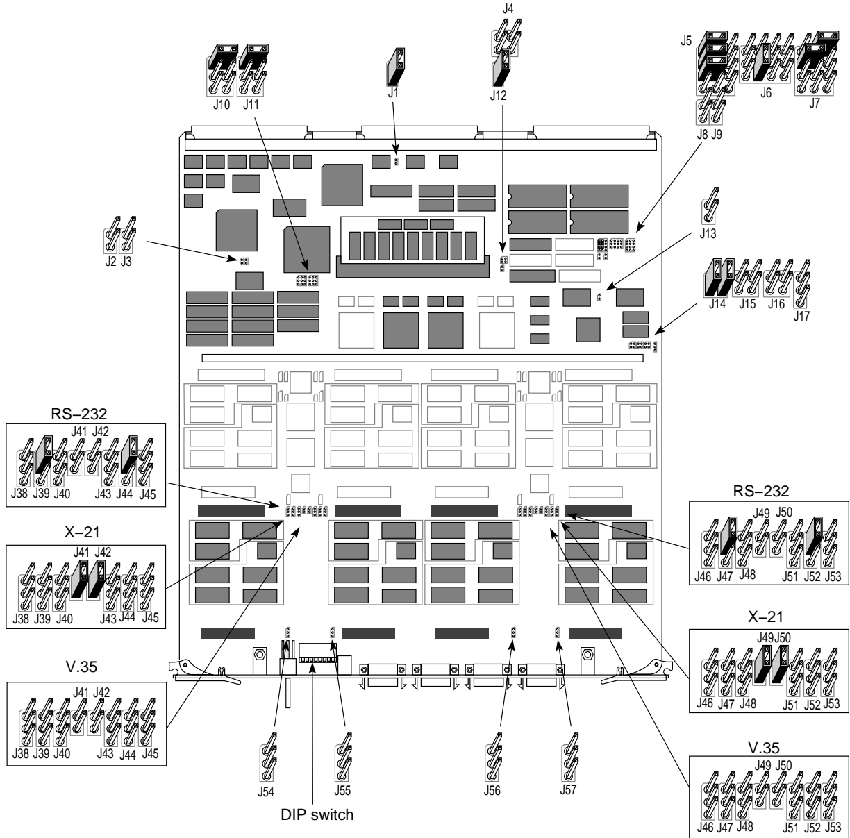
Figure 2-2 VME Sync Board With Required Jumper and DIP Switch Settings (Board 0 Configuration Shown)
