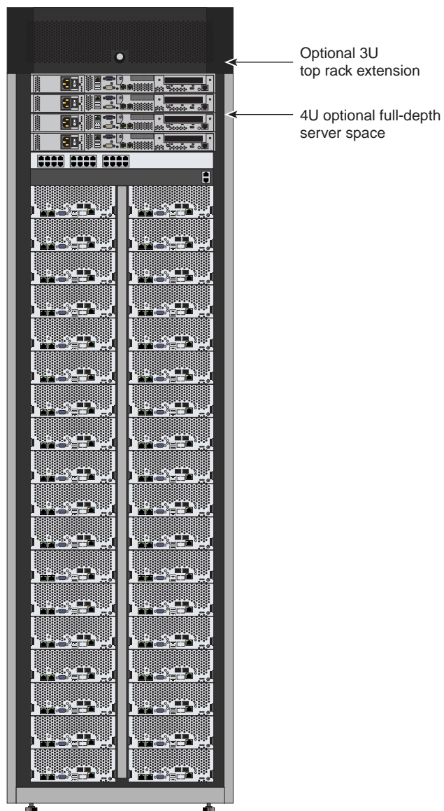
Figure 1-2 Hadoop Specialized InfiniteData Rack Option Example
