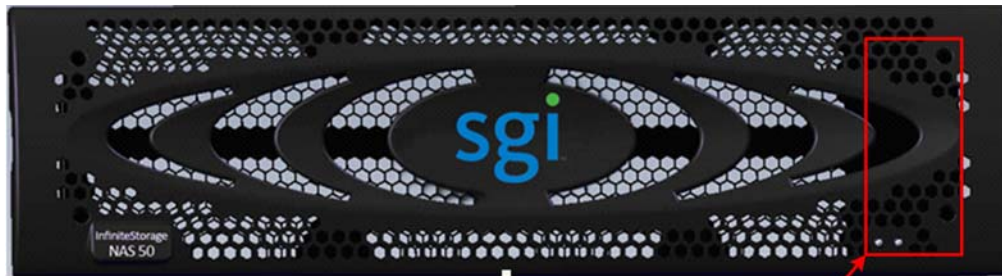
NVRAM Battery Backup Pack (behind front fascia)
