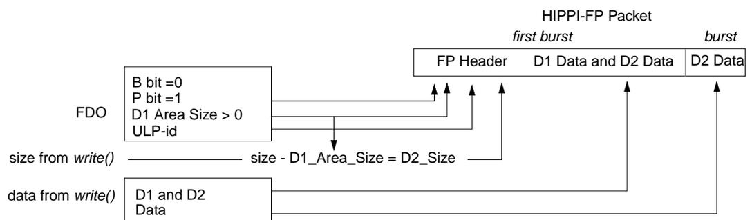
**Figure 1-8** Single-Write HIPPI-FP Packet With D1 Data
