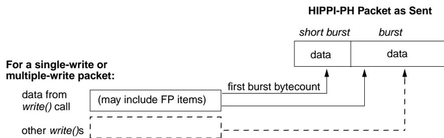
Figure 1-5 Creation of HIPPI-PH Packet With First Short Burst
