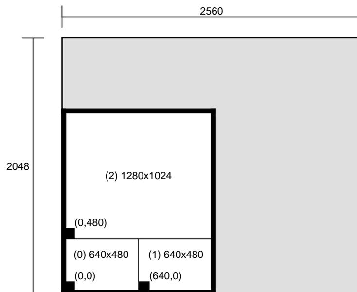
**Figure 2-2** Display Surface for 2@640x480\_60+1@1280x1024\_60
