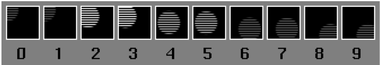
Figure 4-3 Line Doubling on a Single Field
