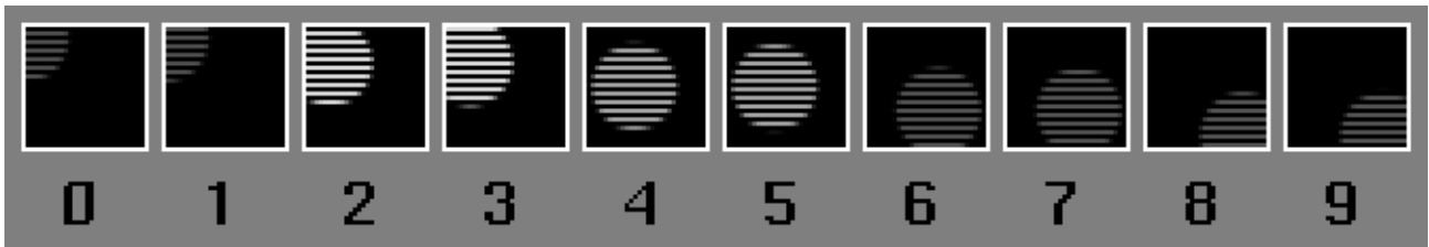
Figure 2-6 Video is not Pairs of Fields of Identical Images With Alternate Scanlines
