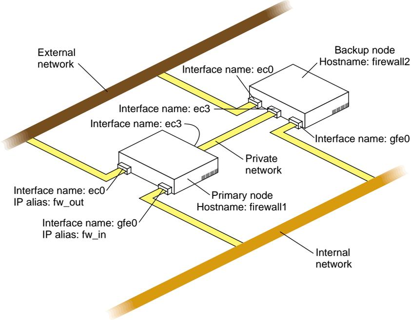
Figure 1-1 Example IRIS FailSafe Gauntlet Configuration
