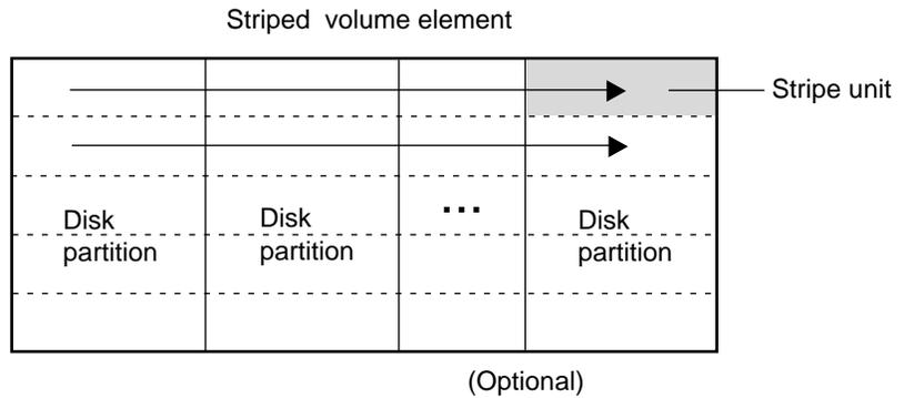
**Figure 4-6** Striped Volume Element Composition
