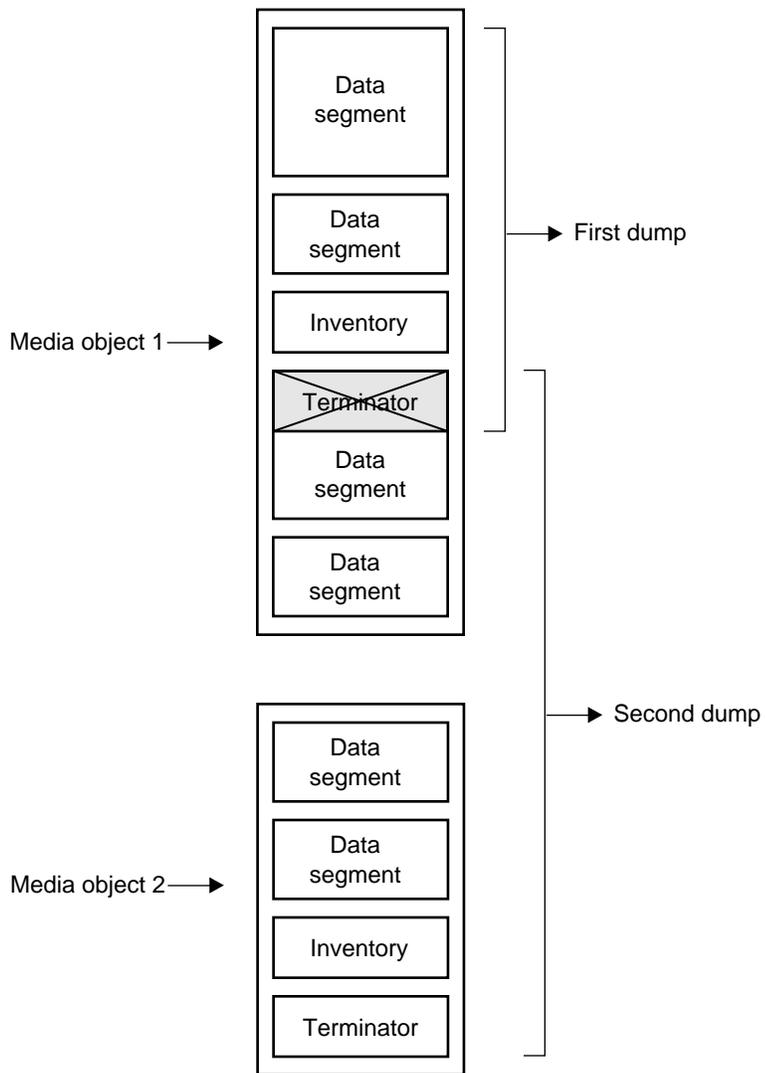
Figure 3-4 Multiple Dumps on Multiple Media Objects
