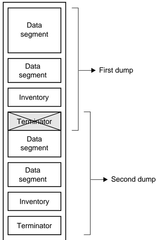
**Figure 3-3** Multiple Dumps on Single Media Object
