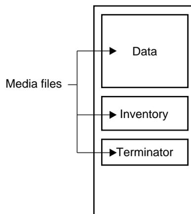
**Figure 3-1** Single Dump on Single Media Object
