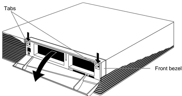
**Figure 1-4** Removing the Front Bezel from the Indigo<sup>2</sup> Chassis
