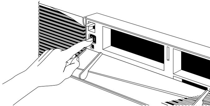
**Figure 1-2** Pressing and Releasing the Power Switch
