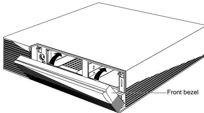
**Figure 3-2** Replacing the Front Bezel on the Indigo<sup>2</sup> Chassis
