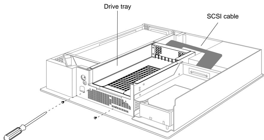
**Figure 2-2** Removing the Screws on the 5-1/4" Drive Tray
