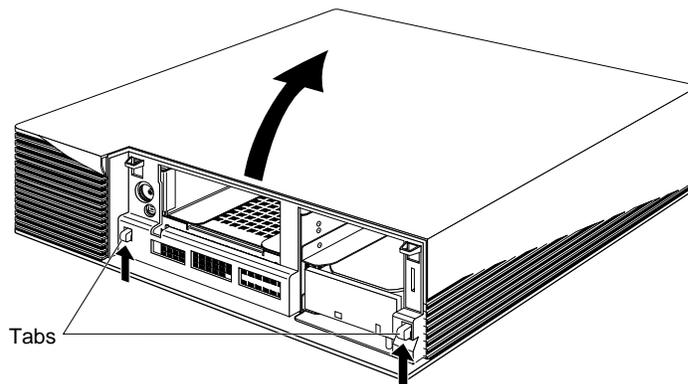
**Figure 1-5** Removing the Top Cover of the Indigo<sup>2</sup> Chassis
