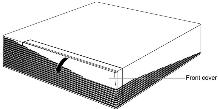
**Figure 1-1** Opening the Front Cover of the Indigo<sup>2</sup> Chassis
