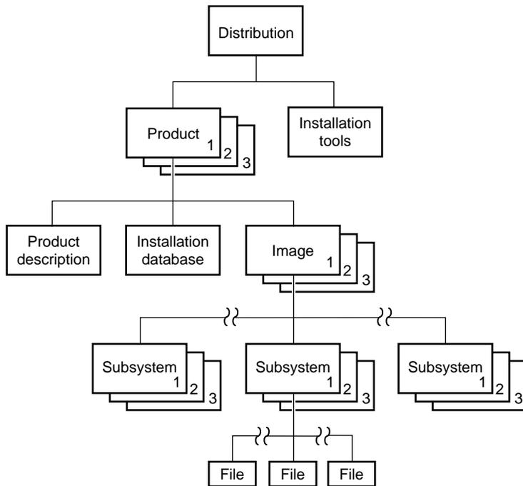
Figure 1-1 Components of a Distribution
