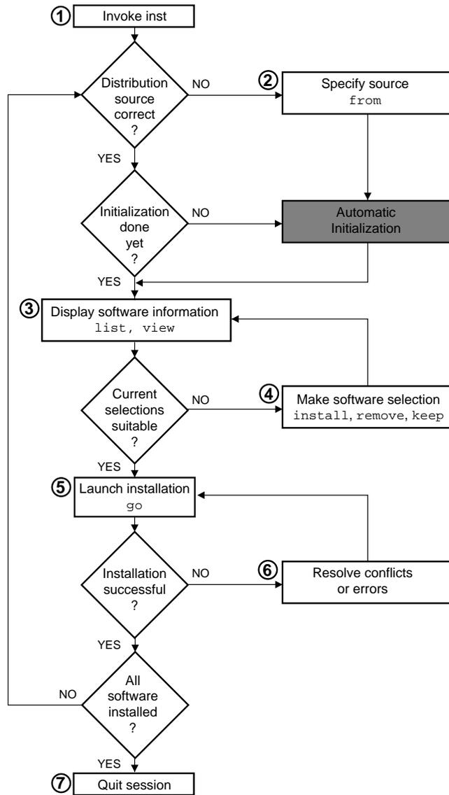
Figure 5-1 Summary of the Installation Procedure
